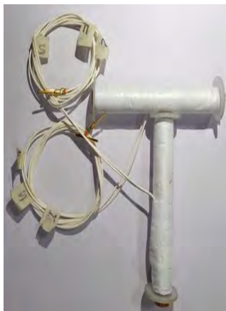
Figure: Magnetotorque and Single axis Momentum wheel based ADCS system developed at IIST by M Tech Control Systems students.
