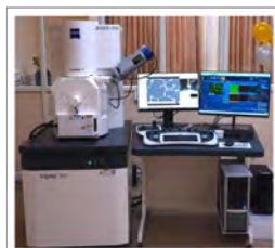
Field Emission Scanning Electron Microscope (FE-SEM) Model: Zeiss Sigma 360
