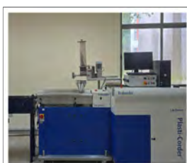
Twin Screw Extruder Model: Brabender
