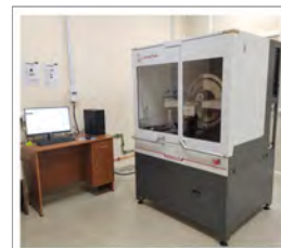
X-ray Diffractometer (XRD) Model: Anton Paar XRDynamic 500
