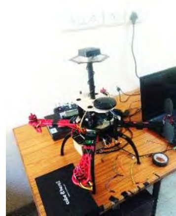
Figure: Magnetotorque and Single axis Momentum wheel based ADCS system developed at IIST by M Tech Control Systems students.
